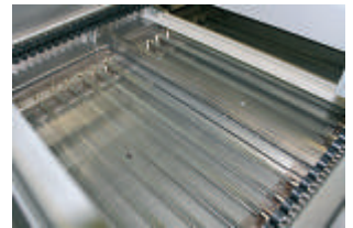
infrared preheat zone
